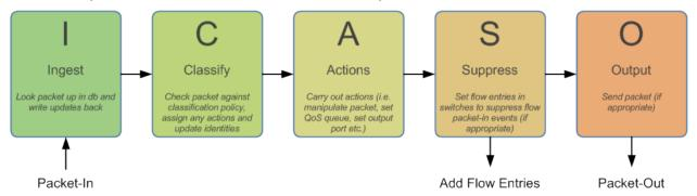
Nmeta configures a single flow table per switch with a table-miss flow entry (FE) that sends full unmatched packets to the controller. As flows are classified, specific higher-priority FEs are configured to suppress sending further packets to the controller.
