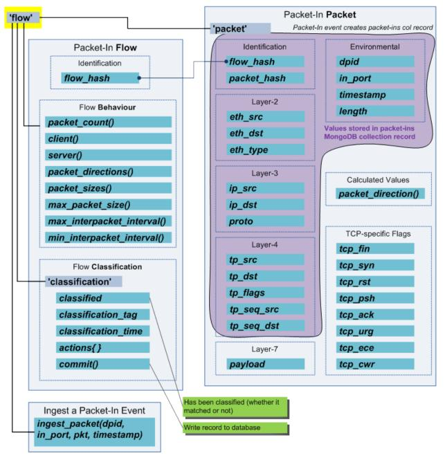
Classifiers can make use of the flows object to gain easy access to features of the current flow.
