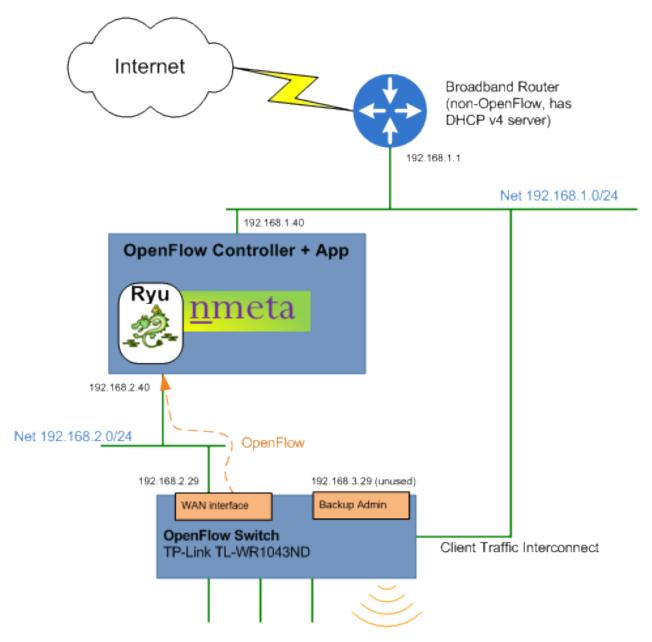
Wired and wireless clients connected through OpenFlow switch (on 192.168.1.0/24 subnet)
